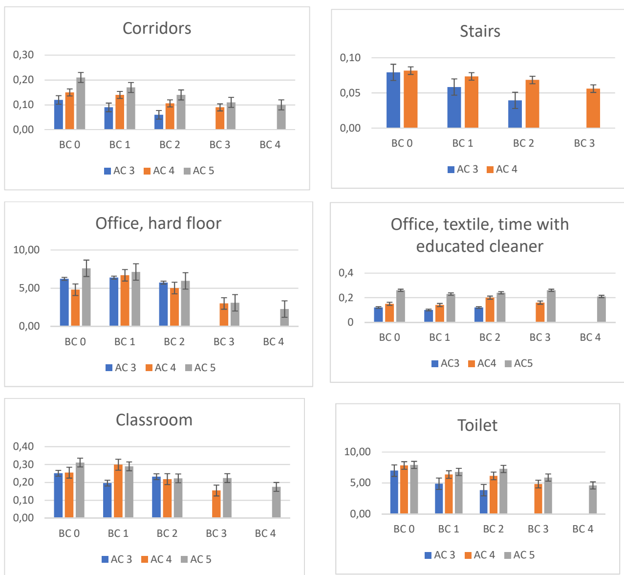
Figure 9. Time dependence on the amount of dirt before cleaning (BC) at different quality levels after cleaning (AC). The numbers refer to quality levels in the INSTA standard. Times are shown in min/m 2 , except for offices with hard floors and toilets in min/room.
