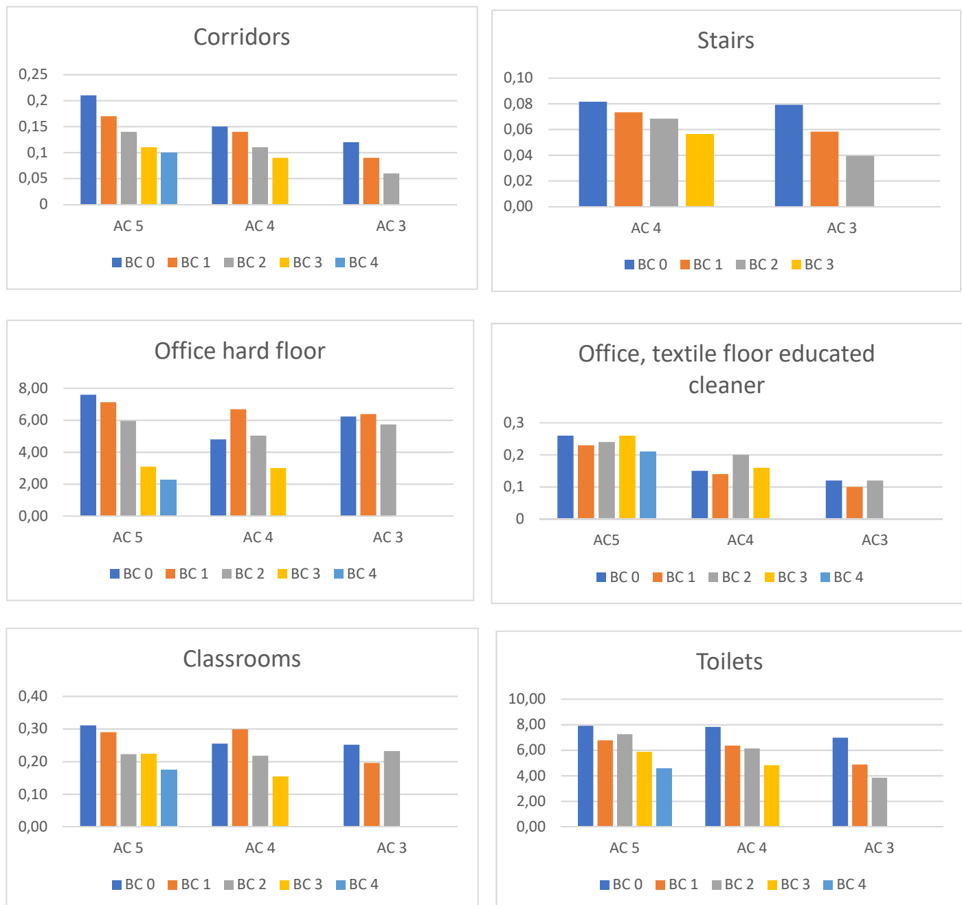
Figure 11. The effect of set quality level in different soiling situations is show in the figures below. Times are shown in min/m 2 , except for offices with hard floors and toilets in min/room.
