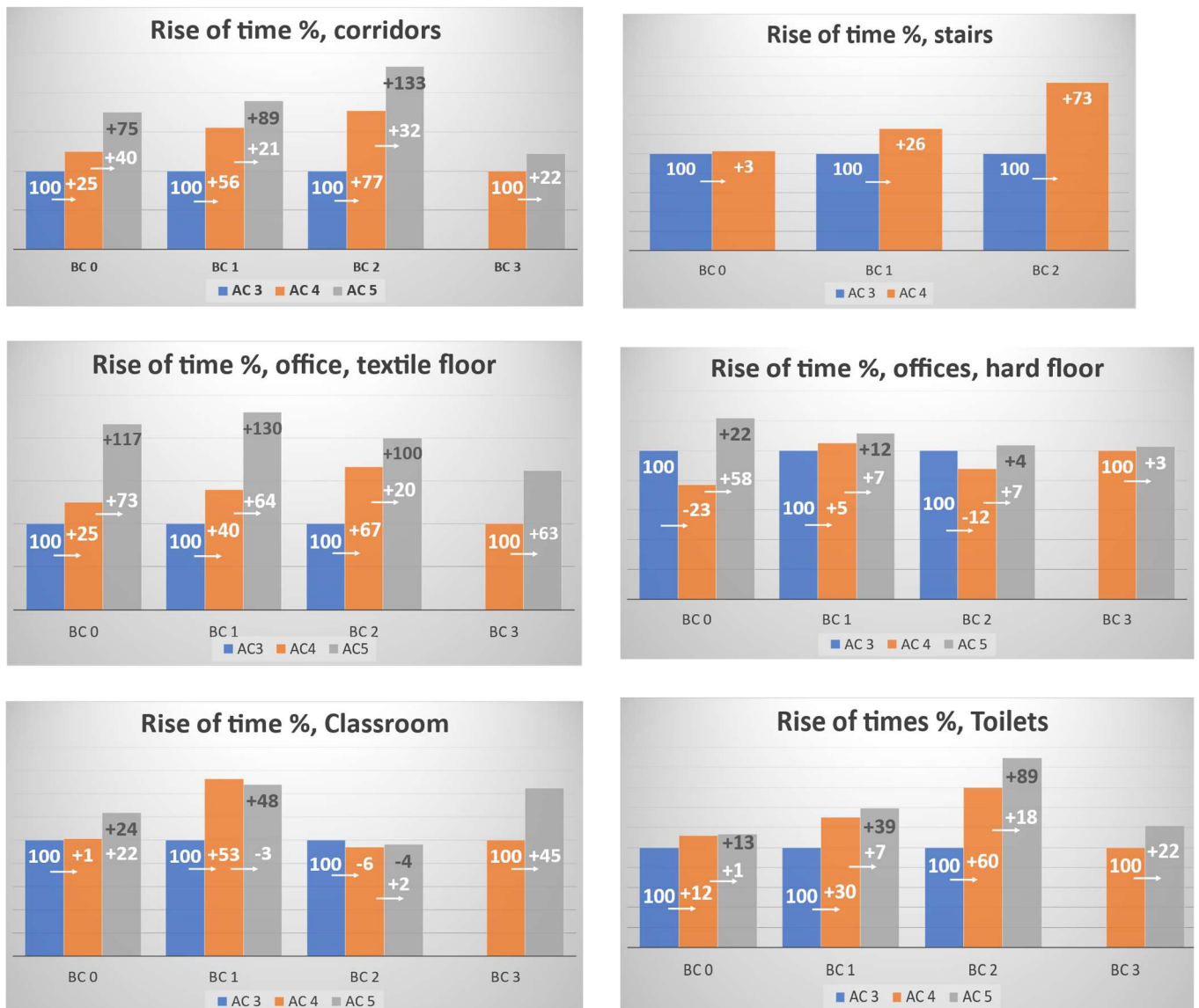
Figure 10. Rise of time as percentages in different room types and at different soiling levels before cleaning (BC) and quality levels after cleaning (AC). The number after BC and AC refers to INSTA 800 standard quality levels. Percentages in white font represent the rise as the quality level increases by one. Percentages in black font represent the rise compared to quality level 3 after cleaning.
