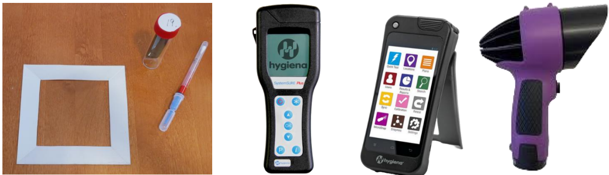
Figure 4. Devices used in tests: ATP and Hygicult devices and UV lamp.
