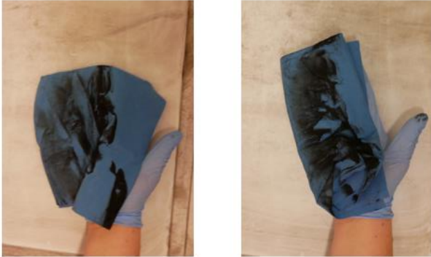
Figure 6. Microfibre cloth folded to four parts (on the left) and six parts (on the right).
