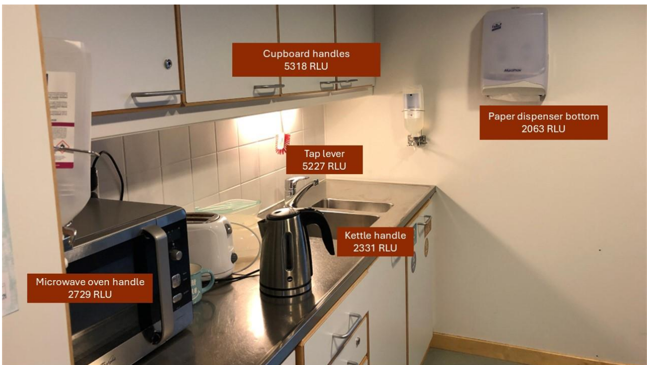
RLU values in an elderly care home staff break room before cleaning.
